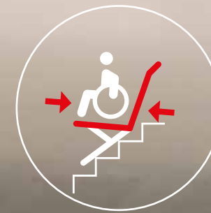
Automatic tilt of the wheelchair
